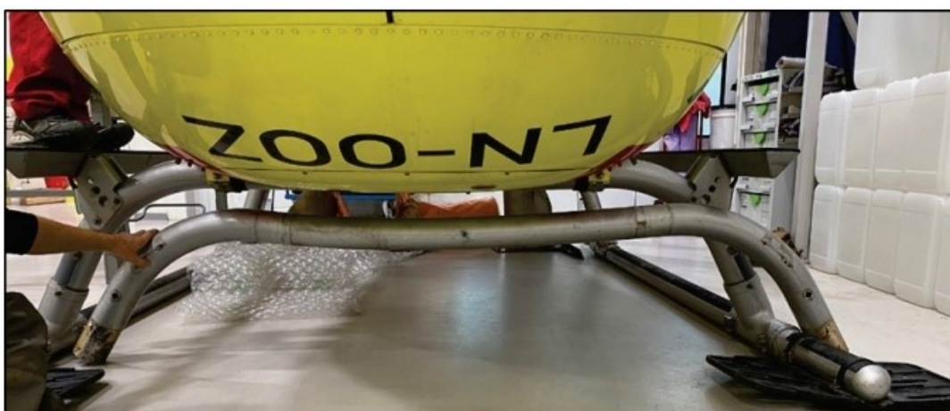
Picture no. 3 – Removed damaged aft crossbeam compared to new installed. The square black rubber plates mounted on the lower aft part of each skid are known as bearpaws.
